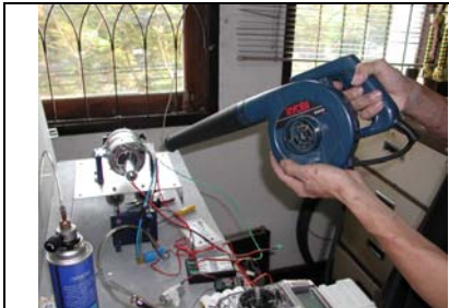
Bench start and blower for added safety and extra cooling
